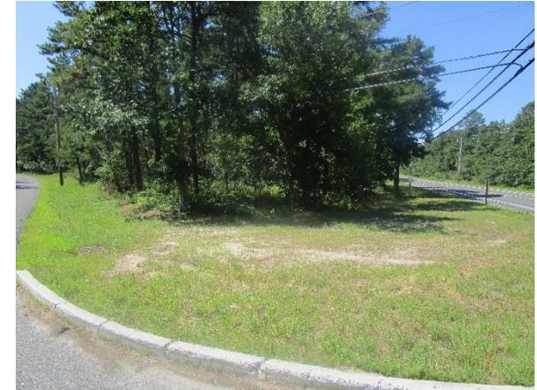
A bioretention system can be installed in the turfgrass area next to the intersection of Panama Road and County Road 563. The bioretention system will capture runoff from the impervious road and will allow infiltration of the runoff instead of runoff directly entering the nearby catch basin. A preliminary soil assessment suggests that the soils have suitable drainage characteristics for green infrastructure.
