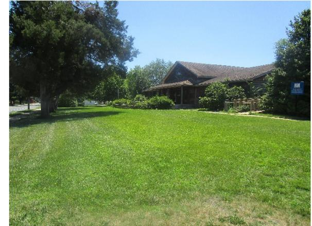
Bioretention systems can be installed in the turfgrass areas at each corner of the municipal building to capture runoff from the roof of the building as well as provide aesthetic value. Pervious pavement can be installed by replacing a section of the parking spaces near the edge of pavement to capture and infiltrate stormwater from the surrounding pavement. A preliminary soil assessment suggests that the soils have suitable drainage characteristics for green infrastructure.
