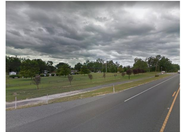
A bioswale can be installed in the right of way in the patch of grass between the road and sidewalk. The bioswale will catch runoff from the impervious road before entering a catch basin. This would convey stormwater in a controlled manner while also removing pollutants and allowing infiltration. A preliminary soil assessment suggests that the soils have suitable drainage characteristics for green infrastructure.
